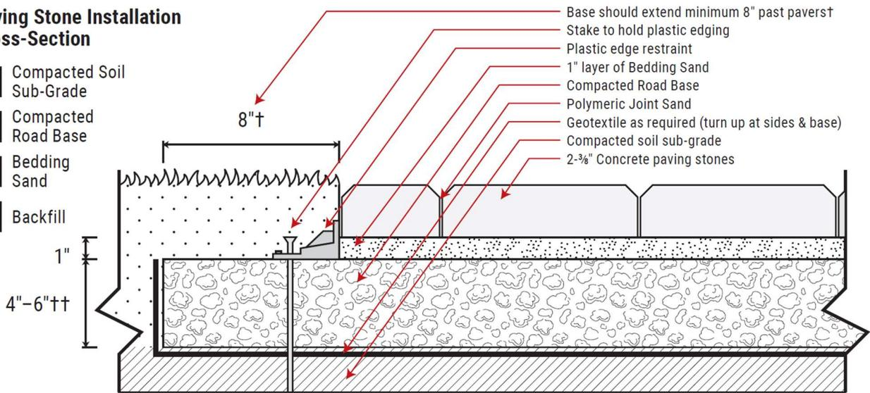
† Extend base by 12" past pavers for driveway installations †† Base thickness should be 8"-14" for driveway installations (depending on underlying soil conditions)
